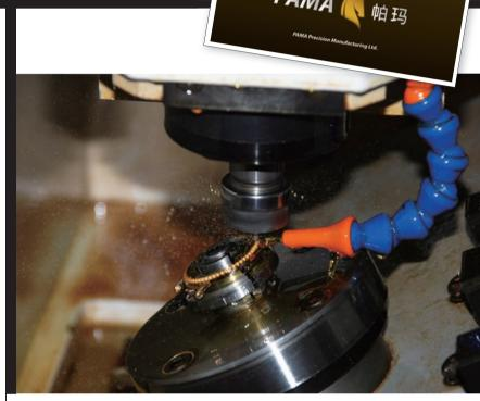
Hardening and brightening of platinum is another leading technology by PAMA. Because of the rarity and special characteristics of platinum material, only a few of manufactures are willing to get involved in this field. As a company specializing in precious metal manufacturing, PAMA has made significant research in the development of platinum products, and successfully developed advanced platinum hardening and brightening technology on its own.
